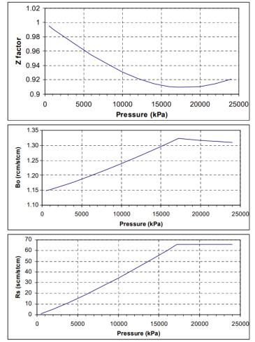
(a) Based on these graphs, what is the bubble-point pressure of this reservoir (to the nearest 1000 kPa)?
